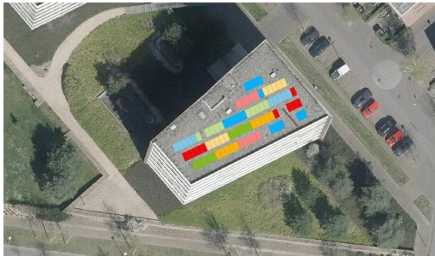
Figure 3: The solar panels grouped per inverter for each apartment
